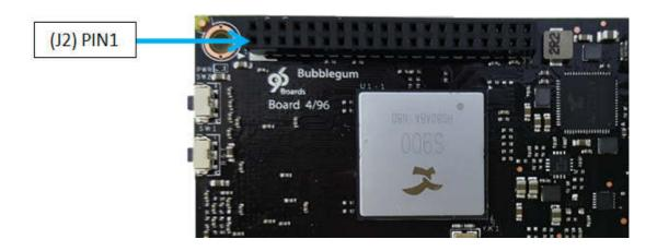
The following tables show the Low Speed Expansion Connector pin out:
