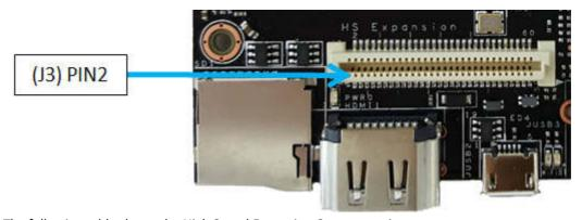
The following table shows the High Speed Expansion Connector pin out:
